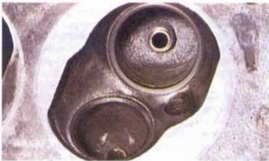
18 When the valve is properly lapped in, the seat should show a thin, unbroken grey line around its circumference as illustrated
