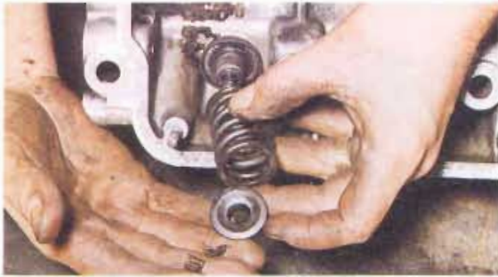
13 From each valve, remove the collets, the spring retaining cap, and the spring. Keep all the components together for re-assembly
