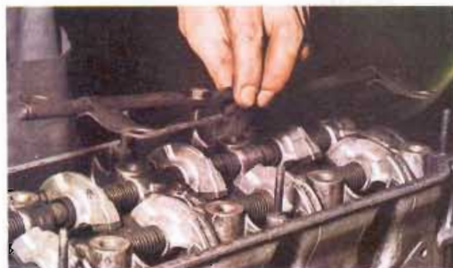
2 Undo the single mounting bolt through which the oil is pumped and lift the oil sprayer bar away from the cylinder head
