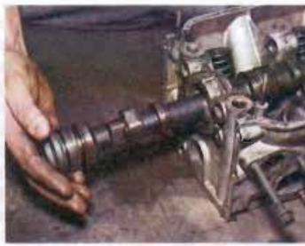
10 With both of the shafts removed, the camshaft can be withdrawn from its three bearing bosses by pulling it away
