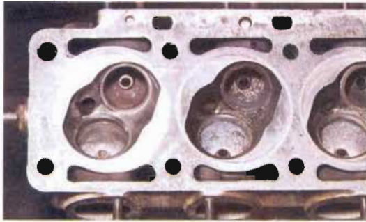
16 When properly cleaned, the combustion chambers should look like the one on the left. Compare it with the uncleaned chamber
