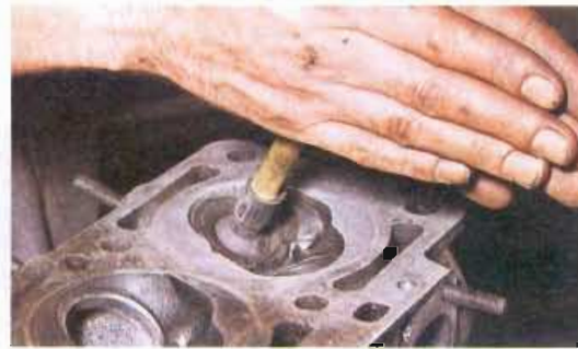
17 Using the correct grade of grinding paste, carefully lap the valves into their seats. Patience is required for this operation
