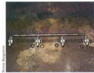
9 To ensure that all the parts are replaced in the correct order, lay out each shaft with all of the relevant components as illustrated
