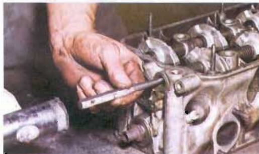
6 Using a suitable drift, carefully drive the rocker shafts from their interference fit housings in the cylinder head casting
