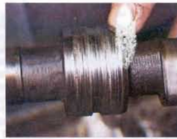
11 Carefully examine the three journals for wear. If any of them are as bad as this, the shaft will have to be replaced
