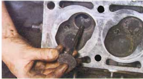
14 Withdraw the valve from its guide and, as you do so, check the sideways play of the valve stem to assess the wear in the guide
