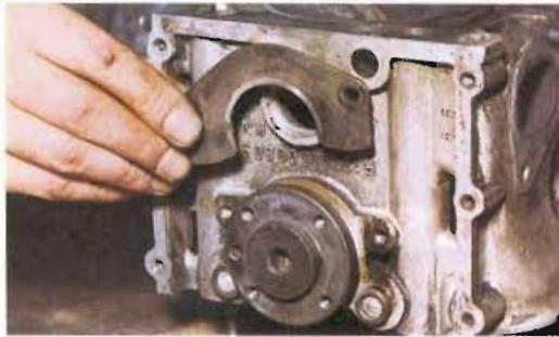
5 With the plug out of the way, undo the two bolts that mount the camshaft retaining plate to the head and lift it away
