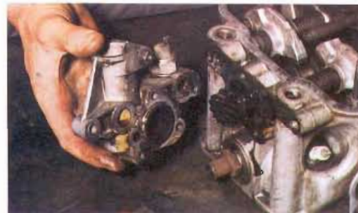
3 When all of the mounting bolts have been removed, lift away the distributor drive housing from its mounting on the head
