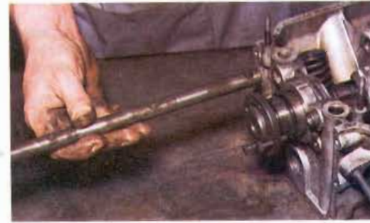
8 When the shaft is almost out of the cylinder head and all of the rocker components have been removed, withdraw the shaft
