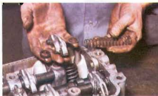
7 As the shaft is driven through each housing, remove the spring, the thrust washer, the rocker and the rubber seal in that order
