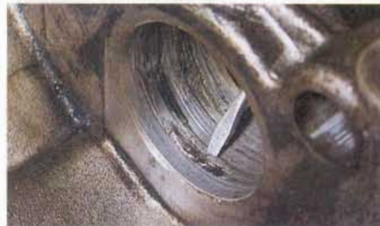
12 Similarly, check the bearing journals in the head. A worn journal such as this can be built up and then machined
