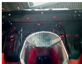
Clockwise from above Refinished underside gains new heat shielding; bodyshell looks like new in shiny red, with all rust surgically removed; engine needed just a check and a clean.
