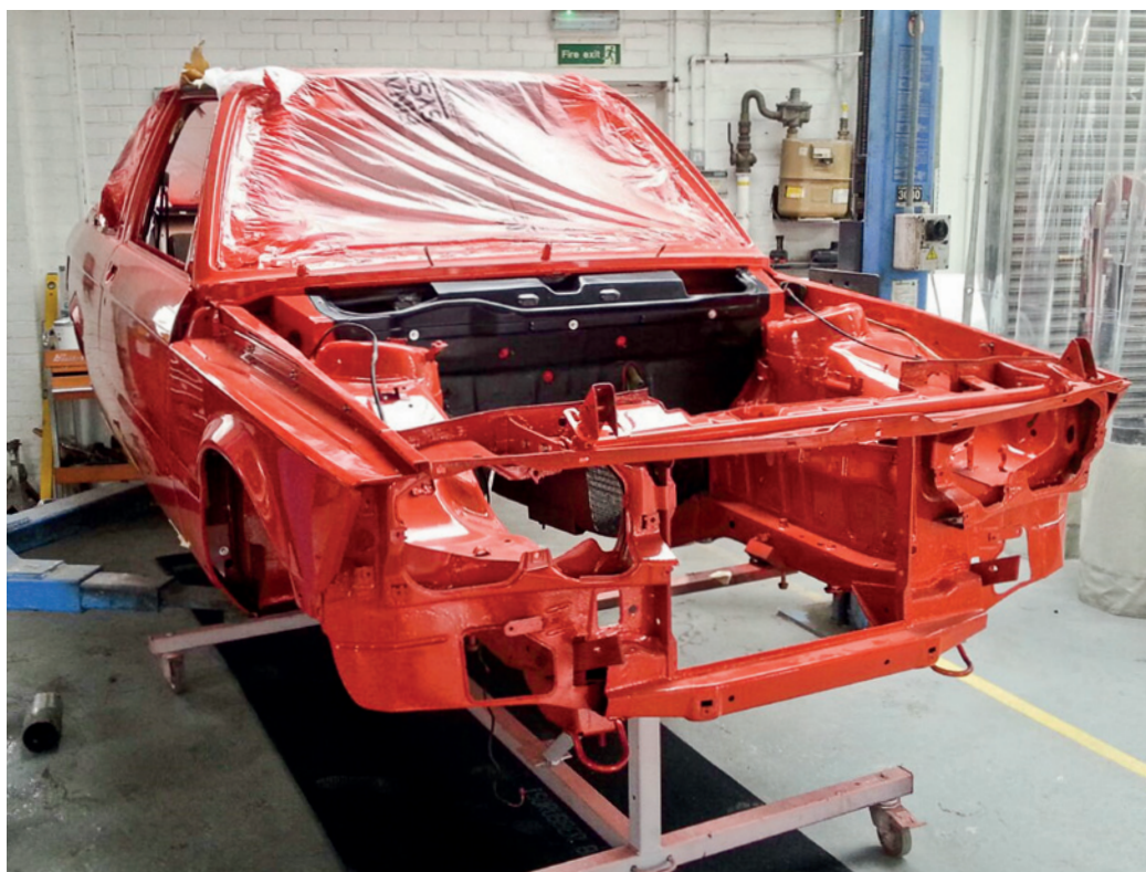
Clockwise from above Refinished underside gains new heat shielding; bodyshell looks like new in shiny red, with all rust surgically removed; engine needed just a check and a clean.
